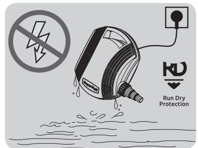
The pump has a thermal overload safety device. In the event of any overheating of the motor, this device automatically switches off the pump. The cooling time is roughly 15 to 20 minutes, then the pump automatically comes on again. If the overload cutout is tripped, it is essential to identify and deal with the cause of the overheating.
